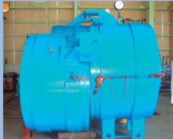
管継手段差200mm Joint height difference 200 mm
