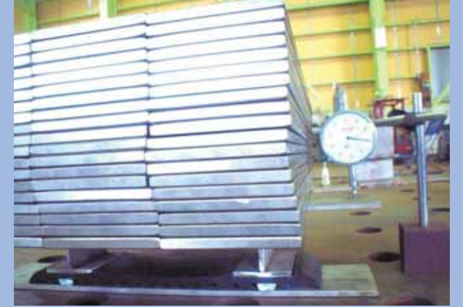
内面バンドゴムの载荷重と圧縮量測定 Internal surface band rubber loading and compression amount measurement
