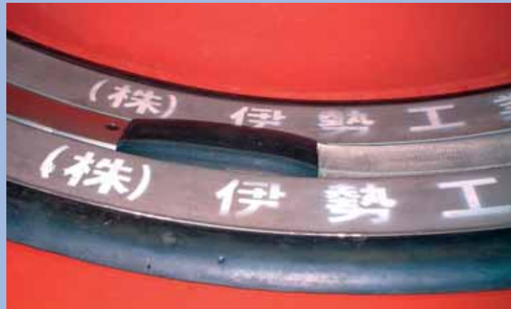
外水圧0.3MPaのゴムと外圧抵抗板 The rubber and external pressure resistance plate under 0.3 MPa external water pressure
