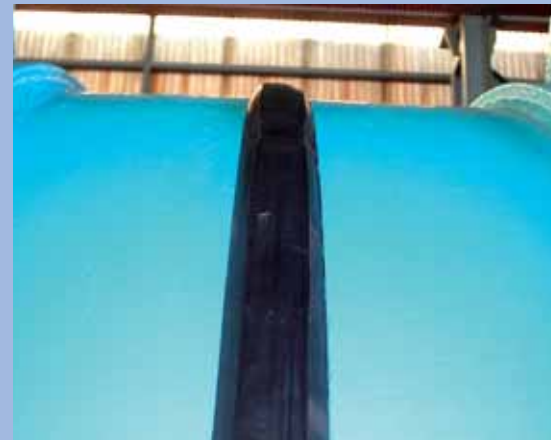
内水圧0.5MPa、継手30mmのゴム膨らみ The rubber inflation of joint length 30 mm under 0.5 MPa internal water pressure
