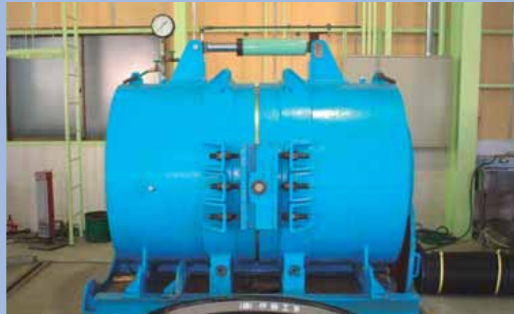
水圧0.8MPa曲げ角3度 Water pressure 0.8 MPa, bending angle 3 degrees
