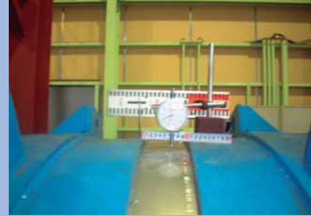
水圧0.8MPa継手間隔100mm Water pressure 0.8 MPa with joint gap 100 mm
